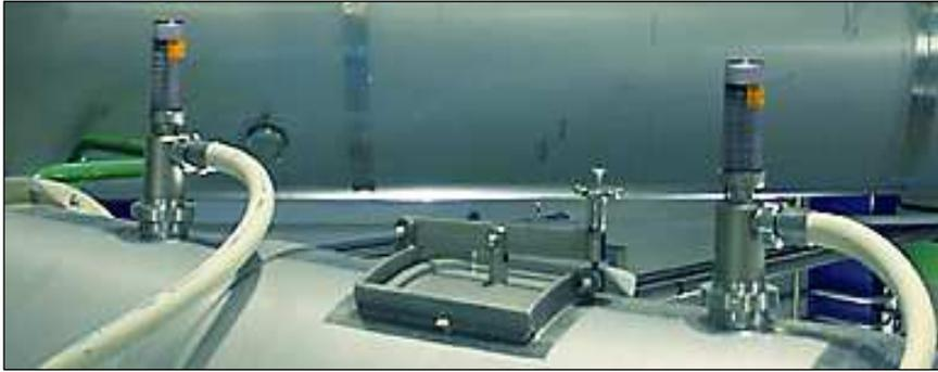
The hoses should be mounted and positioned in such a way so that upon removal of fluid pressure to the CIP Nozzle, the residual fluid can drain back through the hose under gravity and without pooling in any looped sections of hose.
