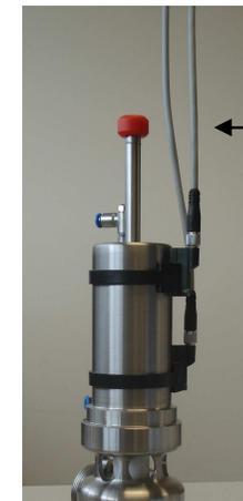
Where there are reed switch indication, a 24V supply needs to be connected to the sensors.
